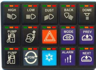
Each button has 3 indicators along the top. These lights report the status of a specific PDM Output for the function of that key.
