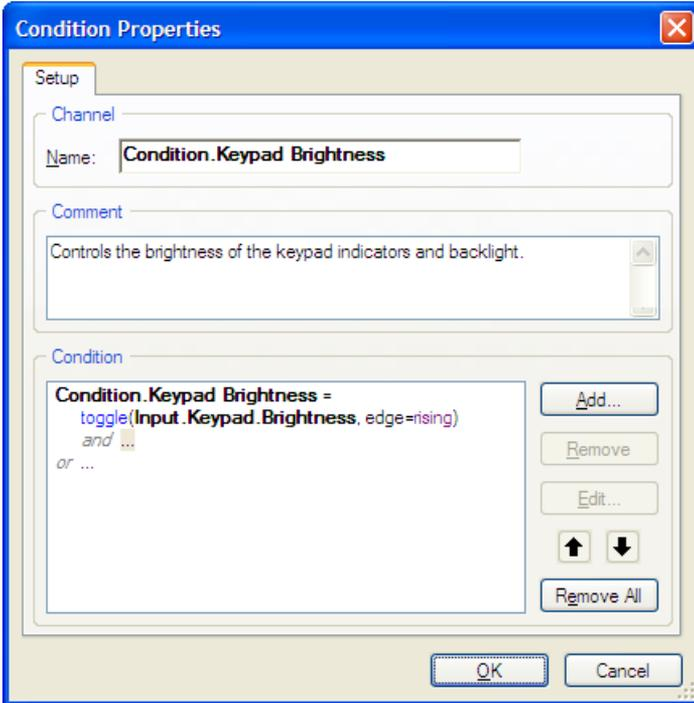
Once this condition is setup, add the channel into the **CAN Outputs** section. See the picture on page 11 where Channel 7 is the brightness channel created from this condition. It is the 8<sup>th</sup> Byte of the second CAN transmission message on ID 0x521 for the first keypad or 0x523 for the second keypad.
