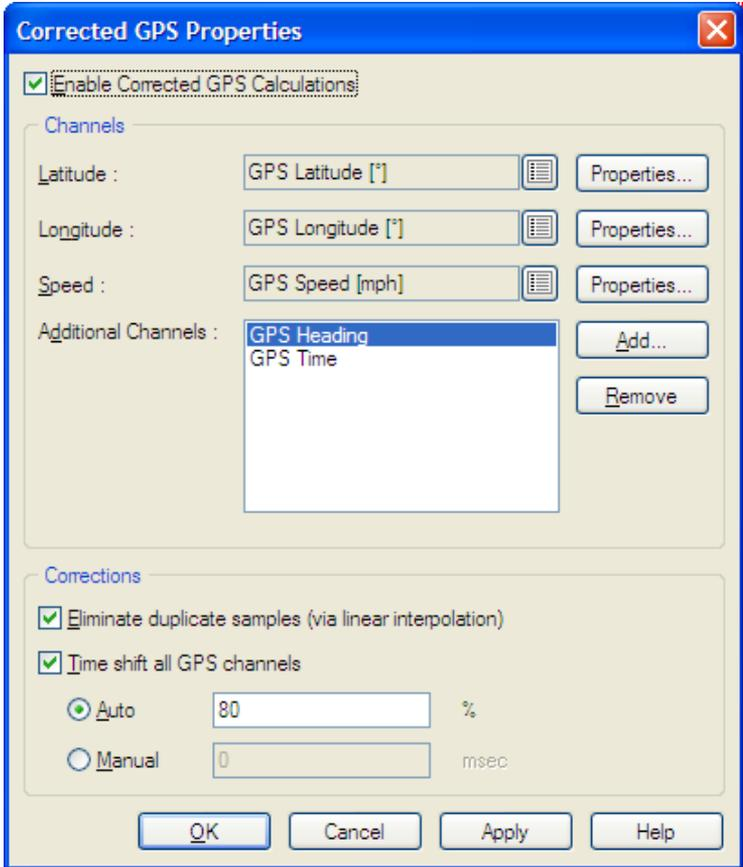
Actual shift may vary. You can use either the Auto function or manually adjust the time delay. The 10 Hz unit typically has a delay of approximately 130 msec. The 20 Hz unit typically has a delay of approximately 110 msec.
