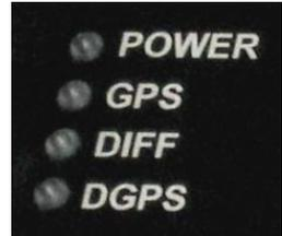
There are only two required lights for operation, one is POWER and the other GPS. The DIFF and DGPS lights indicate increased accuracy of the data. With differential correction, you will get the most accurate data. Therefore best operation is achieved with these lights on.
